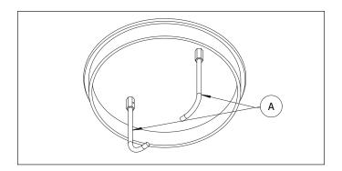
**STEP 7:** Fit the cap onto the bollard, ensuring that the longer axis of the cap aligns with the long axis of the bollard base. Press the cap and the J-anchors into the wet concrete until the cap sits flat on the base.
